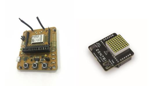
Above, Left: AMW106-E03 (Moray106)Above Right: ASG001 (Monitor board with additional Display)
